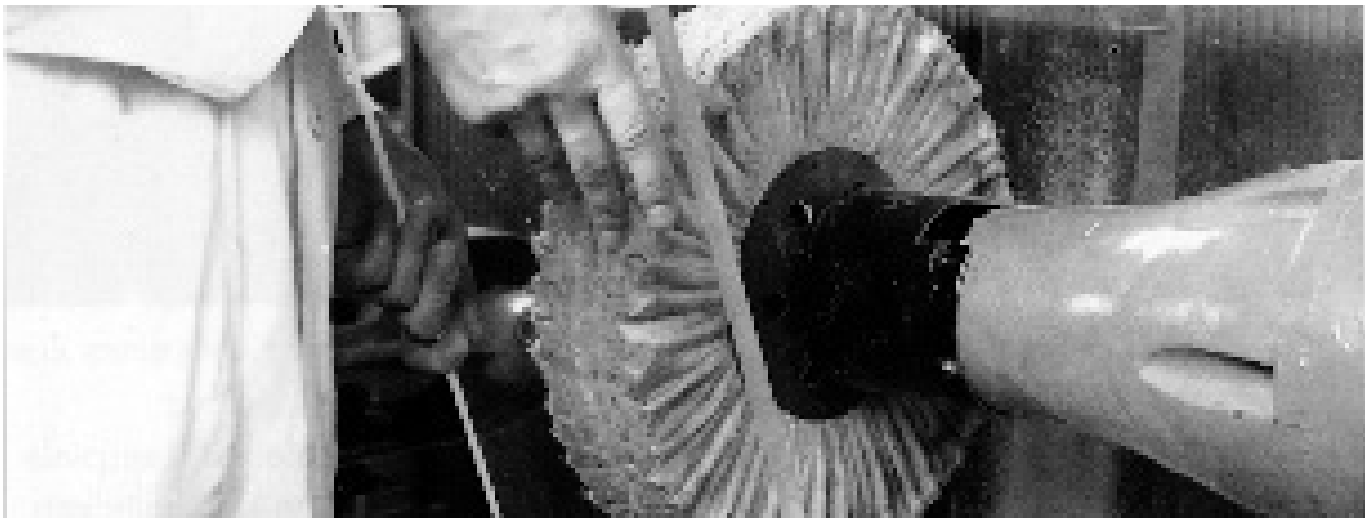
Fig. 40: Polishing against a cloth buffing wheel
