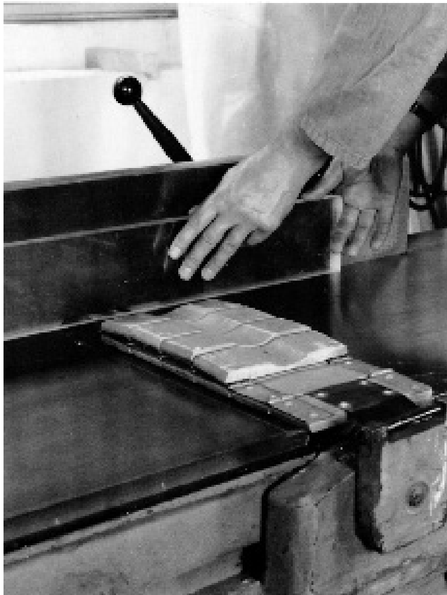
Fig. 36: Smoothing the edges with a surface planer
