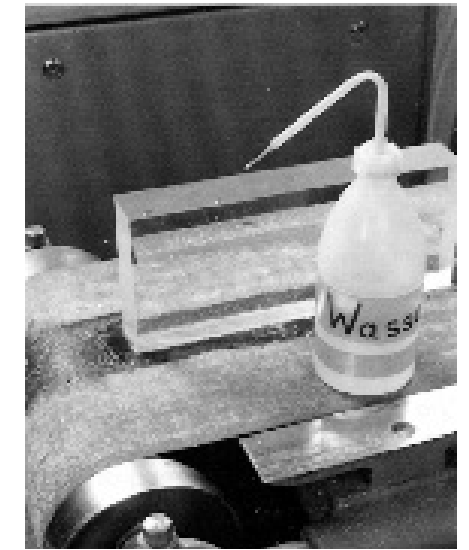
Fig. 38: Wet sanding on a belt sanding machine
