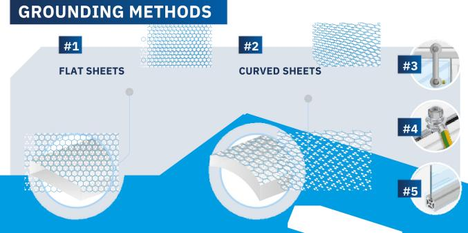
1 Flat panels offer better electro-static dissipation 2 Curved panels offer less efficient electro-static dissipation 3 Potential equipotential bonding by hinge 4 Ground connection Al-profile (ESD) 5 Grounding by panel element
